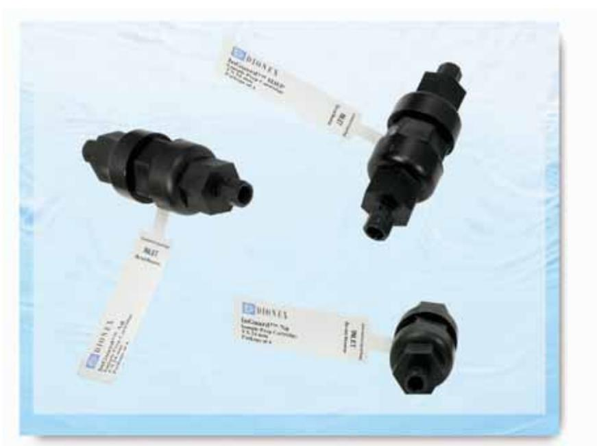
*The InGuard™ line of sample pretreatment cartridges is designed to remove matrix interferences such as cations (including transition metals), anions, or hydrophobic substances that are encountered in many ion chromatography (IC) applications. The InGuard cartridge is installed in-line between the autosampler and the IC injection valve, facilitating immediate, automated sample pre-treatment.*
